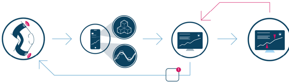
Figure 1. Schematic of the remote patient monitoring platform. First, the knee sleeve transmits basic spatial data to the smartphone during a standard post-operative rehabilitation TKA exercise. Then, the smartphone transmits this data through the artificial intelligence (AI) processor that analyzes the data and immediately returns real-time feedback to the patient regarding number of repetitions, max flexion, or if lacking extension. If the patient does not reach 90° of flexion by two weeks postoperatively, the surgeon is notified.
